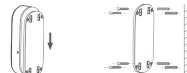
Press against the back of the door bell, and push down to get the back cover.
